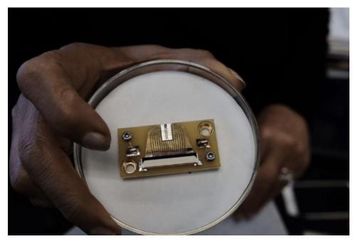
Prof. Razeghi holds the world's first tiny array of tunable infrared lasers that she developed for Department of Homeland Security. A patent is pending for the device, which allows for molecular spectroscopy and is enabling a new generation of airport scanners.
