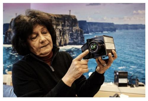
Razeghi displays a high-operating temperature mid-wavelength infrared camera developed in her lab. The camera allows superior infrared imaging in a portable format valuable for a range of applications — from military and national defense use to medicine.
